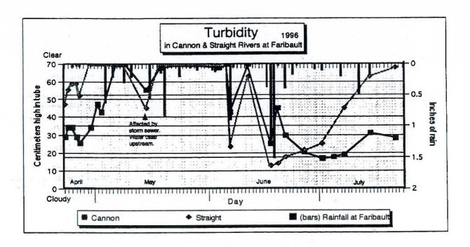
Turbidity tubes are read by pouring water into the tube until a black and white design on the bottom of the tube is obscured. The number of centimeters of water in the tube is then recorded. Cloudy, or turbid, water will obscure the design sooner than clear water.
